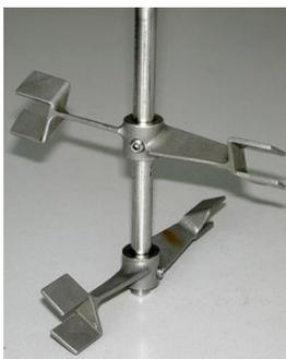
Ekato Intermig is one of the most widespread mixers for mycelial cultures. This type of mixers consists of two mixers - the lower and upper one. In this combination, axial flows are generated in the mixer, and the mixer's radial end construction ensures a sufficient radial mixing. Thereby, an even distribution of the energy introduced by the mixer throughout the bioreactor's volume is ensured, resulting in the decrease of the maximal shear forces.
