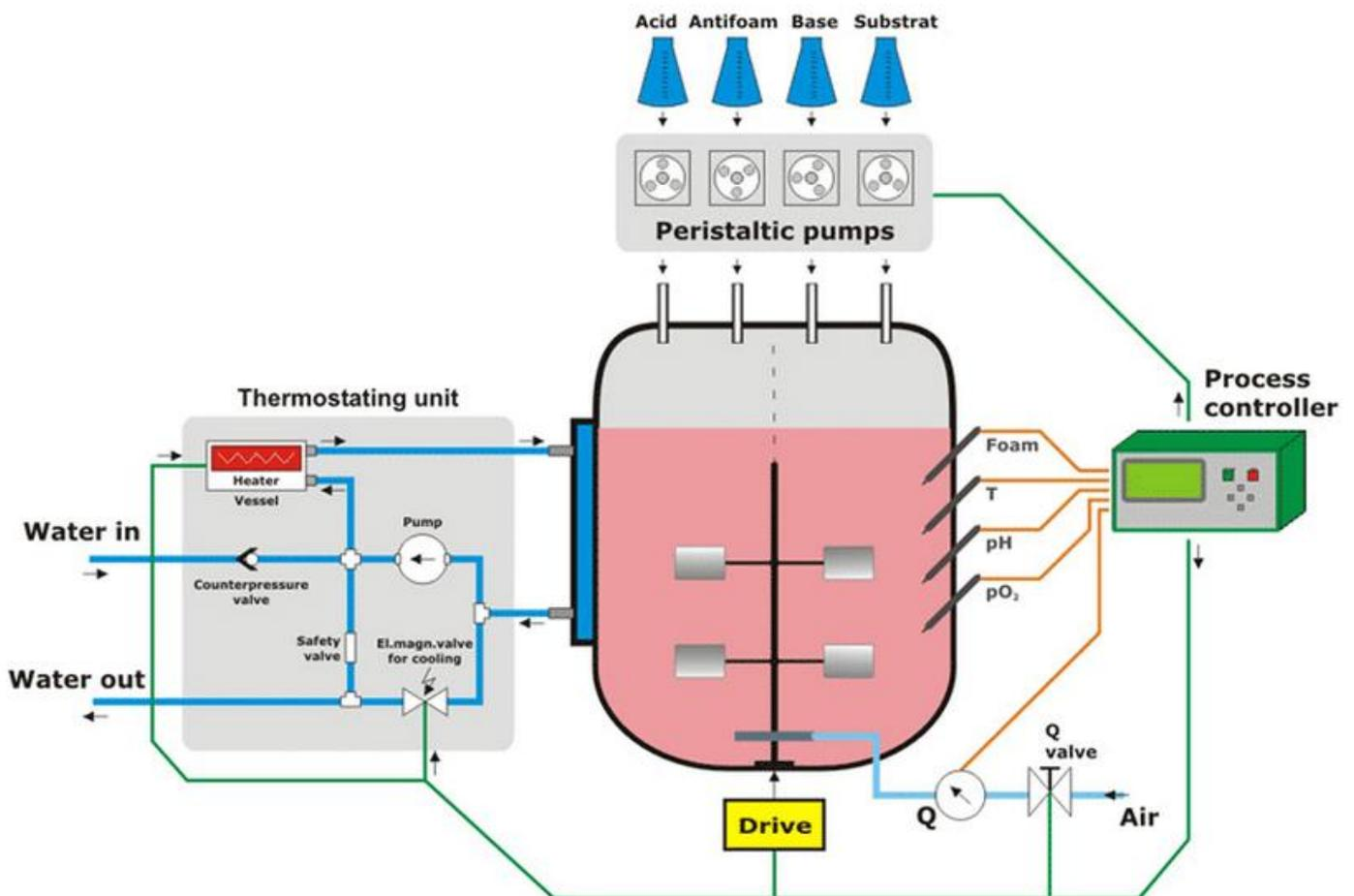
Temperature, pH, pO<sub>2</sub> and foam are the parameters that are usually controlled and monitored in bioreactors.
