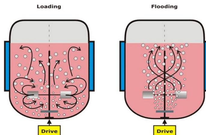
As it can be seen in illustration - as the "flooding" regime sets in, air bubbles are concentrated only in the middle part of the reactor, and they are poorly dispersed. Hence, such a mixing/aeration state is very undesirable for the microorganism growth.
