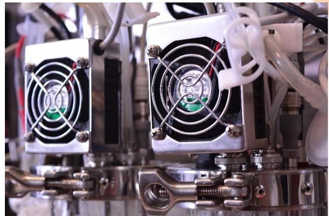
Heating and cooling functions can provide either heating of cooling functions for the glass vessel and can be done independently between both vessels
