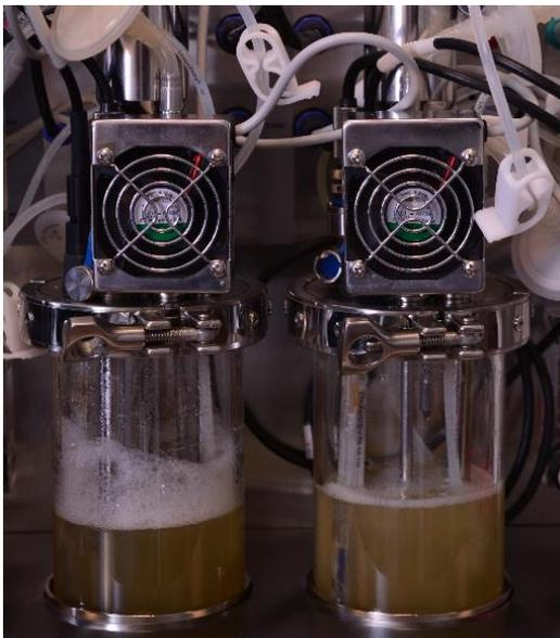
Easily exchangeable, large 1L glass vessels provide the option to use multiple vessels with the same lid providing the flexibility in day to day operation and easing in research production
